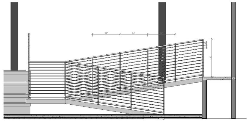
6 CORTE A - DETALHE GUARDA CORPO
